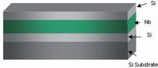
Figure 1. The design of fabricated nano-sized layered structure based on Nb-film.
